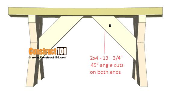
Cut two 2×4's to 13 3/4" long for the bench brace (D), all the ends will have 45 degree angle cuts in opposite directions. Drill pilot holes and attach as shown on illustration above using 2 1/2" deck screws.
