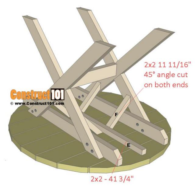
Cut one  $2\times2$  to  $41\ 3/4$ " long for the table brace (E). Cut two  $2\times2$ 's to  $11\ 11/16$ " long for the table brace (F), cut 45 degree angle cuts on all ends in opposite directions. Install as shown on illustration above using  $2\ 1/2$ " deck screws.
