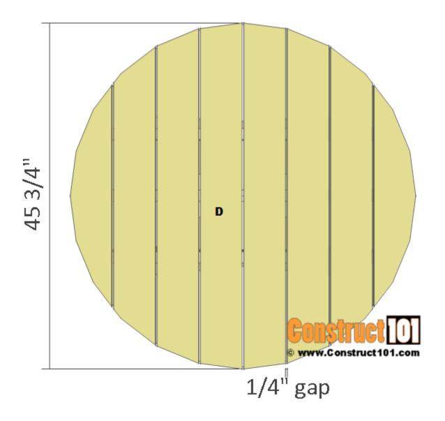
Cut the 2×6 table top planks (D) as shown on illustration above. The easiest way to draw and cut out the circle is by using trammels. Drill pilot holes and screw 3" deck screws through the table planks (D) and into the apron (C).
