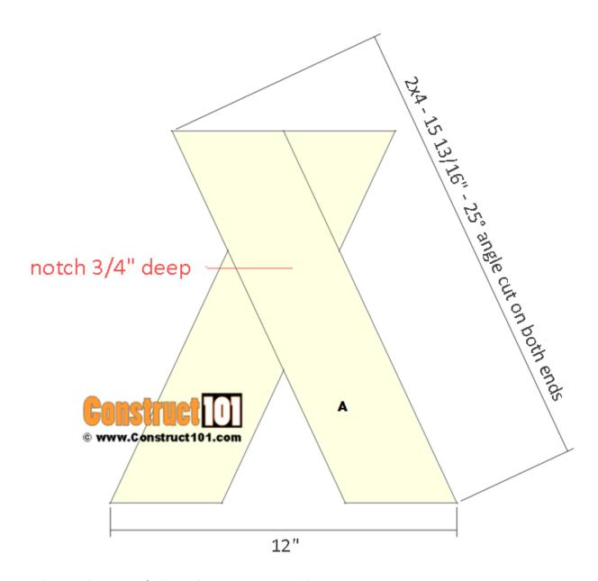
Cut four  $2\times4$ 's to 15 13/16" long for the bench legs (A). Cut the ends at 25 degree angle cut on both ends in the same direction. Drill pilot holes and use 2 1/2" deck screws to attach the legs together.
