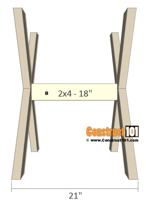
Cut one  $2\times4$  to 18'' long for the stretcher (B). Screw 3'' deck screws through the legs (A) and into the stretcher (B).
