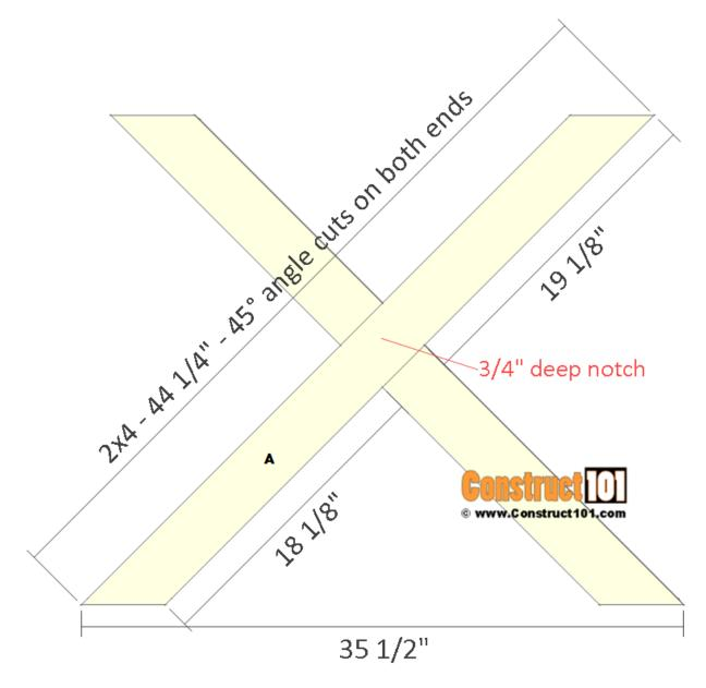
Cut four 2×4's to 44 1/4" long for the legs (A). Cut 45 degree angle cuts on all ends in same direction.
