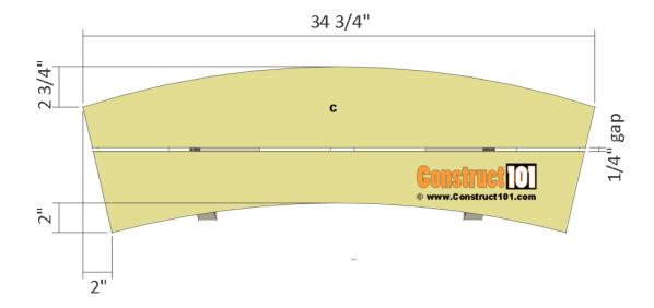
Cut the 2×6 bench seat planks (C) as shown on illustration above. Drill pilot holes and screw 3" deck screws through the planks (C) and into the cleat (B).
