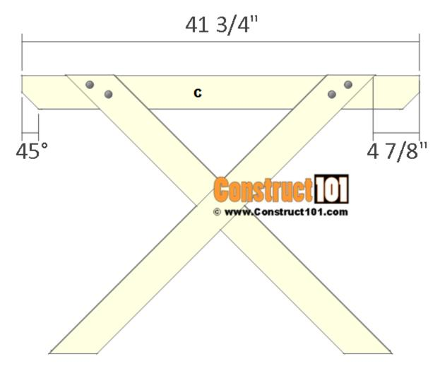
Cut two  $2\times4$ 's to  $41\ 3/4$ " long for the for the table apron, cut the ends as shown on illustration above (C). Attach as shown on illustration above, pre-drill holes and attach with  $3\ 1/2$ " galvanized carriage bolts.
