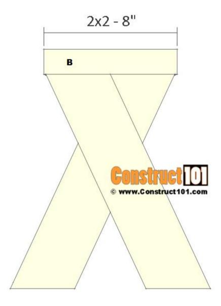
Cut two  $2\times2's$  to 8'' long for the cleat (B). Install as shown above using 3'' deck screws. Drill pilot holes, screw through the cleat (B) and into the bench legs (A).
